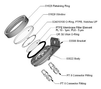
Figure 11-1: Sample Particulate Filter Assembly
